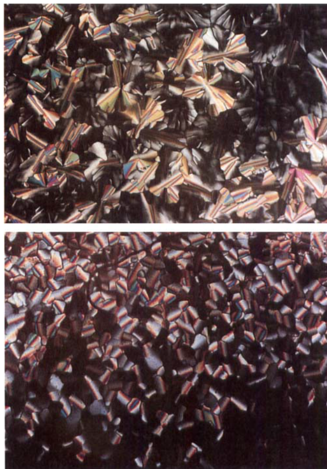
Figure 5. Top: Optical texture of 1b at room temperature (crossed polarisers). Bottom: Optical texture of 1c at 280^{\circ}\text{C} (crossed polarisers).
